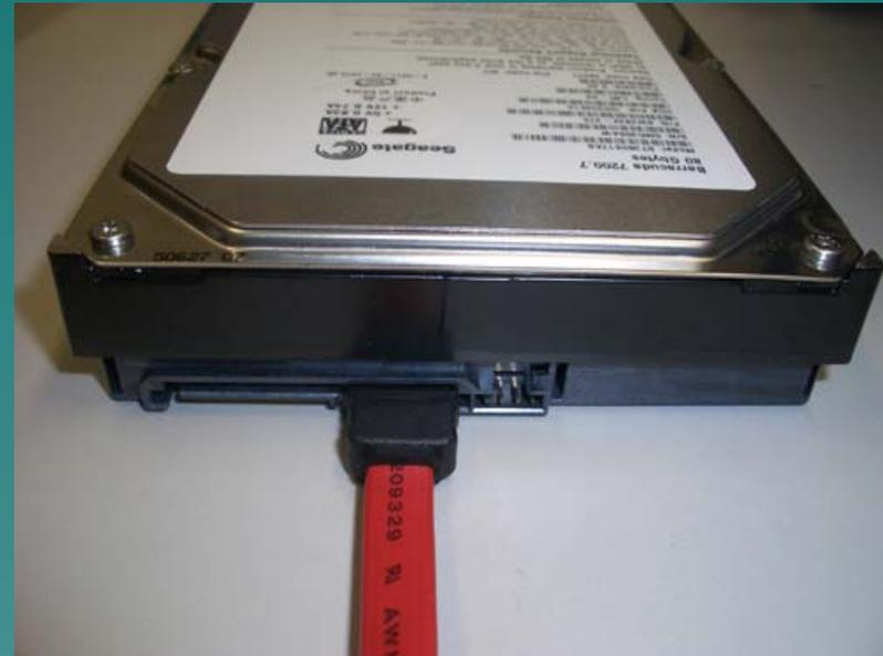
SATA Power cable Connector      SATA Signal cable Connector
